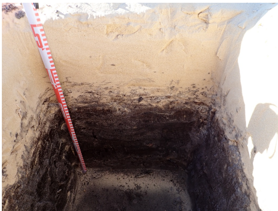
Plate 6: Typical section of a test pit at the base of the dune (DB-TP-04).
